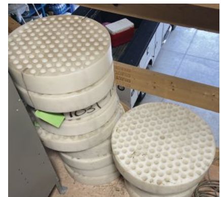
Figure 2. The “cheese plate” assembly maintains the required separation of the ungrouted, noncompacted strands.
