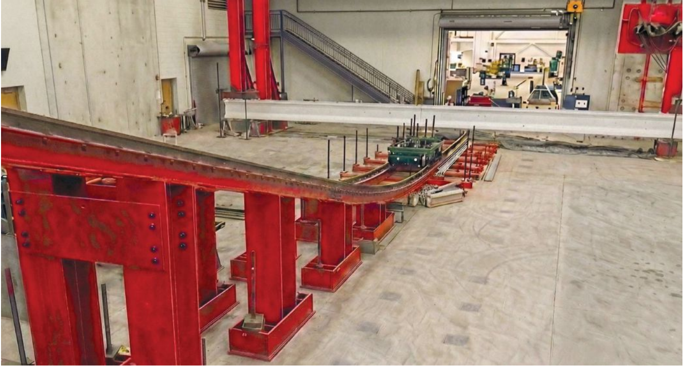
Figure 3. The impact bogie is ready to be released for impact testing of a girder specimen.
