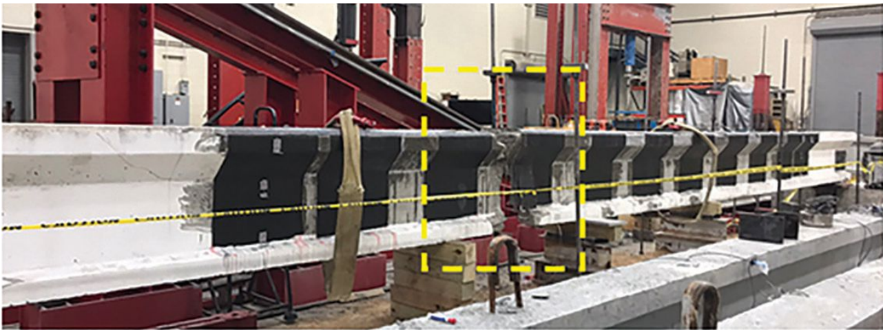
Figure 7. Failure of the carbon-fiber-reinforced polymer (CFRP) repaired girder; only the CFRP-repaired specimens were tested upside down.
