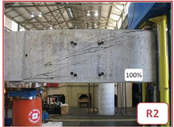
Figure 2. Load deflection behavior of a large-scale reinforced concrete bent cap specimen damaged by alkali-silica reaction (R2) compared with a control specimen (nR1). 3 Figure: University of Texas at Austin.
