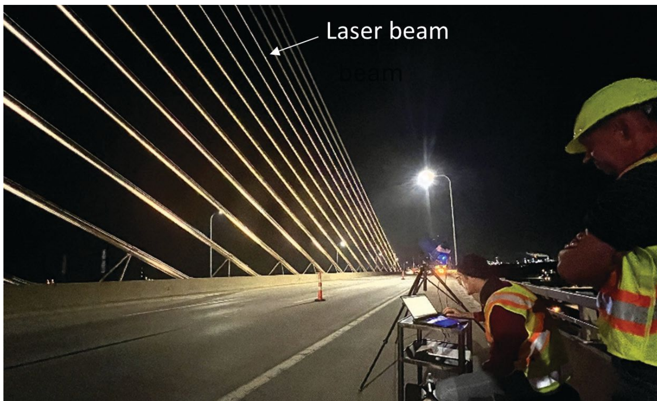
Figure 7. A laser vibrometer is used to collect data from the Veterans' Glass City Skyway deck during a coordinated lane closure to eliminate traffic-induced vibration noise.
