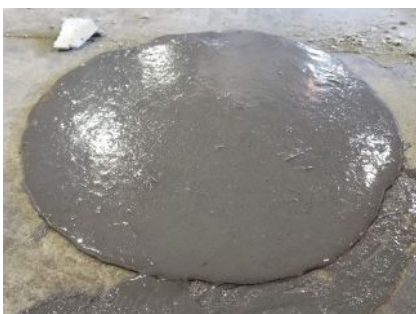
Appearance of ultra-high-performance concrete in its fresh state as it is used for testing (left) and beam production (right). Photos: PCI.
