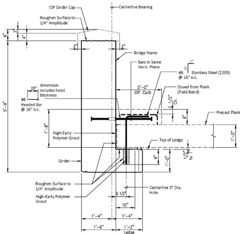
Detail for the typical precast concrete girder-to-slab and girder-to-curb connections. Figure: KSF Inc.
