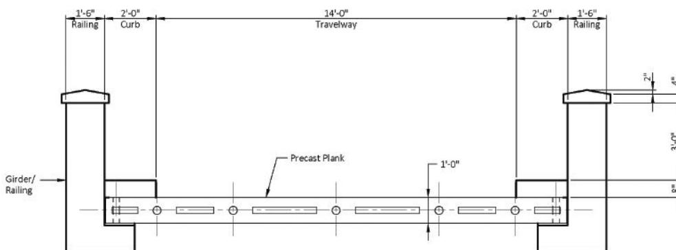
The typical bridge section for the one-lane, 21-ft-wide bridge consists of a 14-ft-wide travel lane, 2-ft-wide curbs, and the precast concrete L-girders that also serve as the bridge railing. Figure: KSF Inc.
