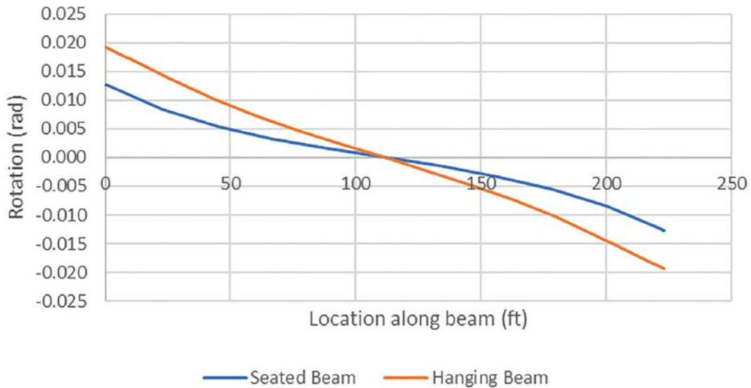
**Figure 2.** Comparison of end rotations of seated and hanging beams for the Puyallup River Bridge girders.
