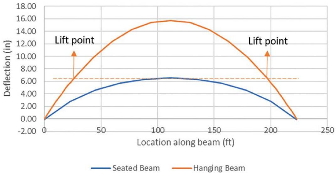
**Figure 1.** Comparison of seated and hanging beam total deflection calculated relative to the ends of the beam using the properties of girders from the Puyallup River Bridge in Tacoma, Wash. All Photos and Figures: Washington State Department of Transportation.
