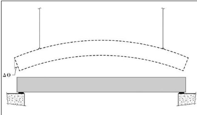
Figure 4. End rotations of a girder in the hanging and seated support conditions.
