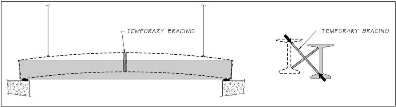
Figure 3. Elevation view of girders showing differential camber at erection and section of adjacent girders showing bracing geometry and forces.
