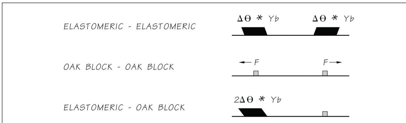
Figure 5. Shear forces and deformations for various bearing support scenarios.
