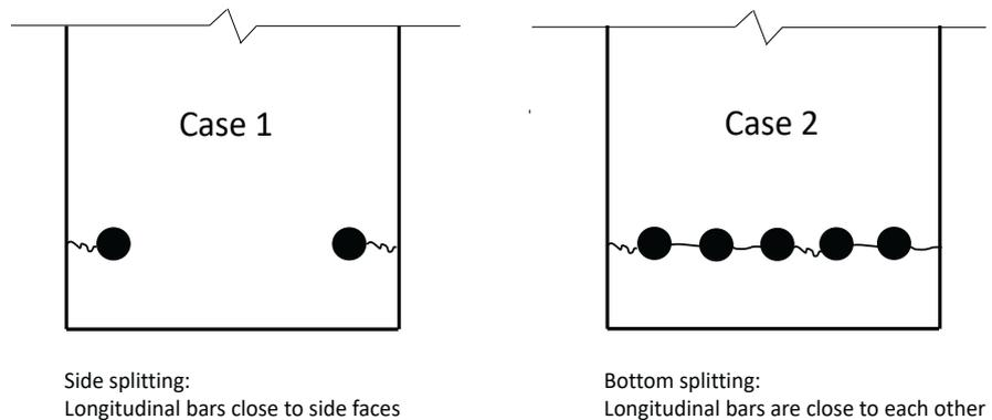
the same limits as Zaborac and Bayrak.<sup>4</sup> To improve the bond strength of no. 11 and larger reinforcing bars in tension terminating in a standard hook, NCHRP Report 603 recommends a minimum amount of transverse reinforcement consisting of no. 3 U-bars at  $3d_b$  spacing in the anchorage length. Similar to the provisions of ACI 318-19, NCHRP Report 603 does not consider hooks to be effective in developing bars in compression.
