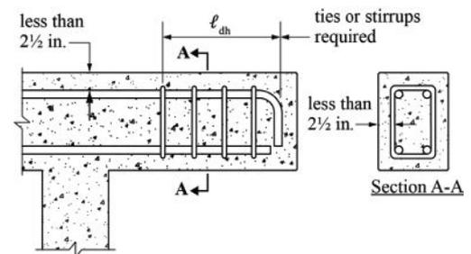
Figure 2. For bars being developed by a standard hook at discontinuous end of components with both side cover and top or bottom cover less than 2.5 in., the hooked bar shall be enclosed within ties of stirrups spaced along the development length  $\ell_{dh}$ . The ties shall have a spacing not greater than  $3d_b$ . Source: Adapted from Fig. 5.10.8.2.4c-1 of the AASHTO LRFD Bridge Design Specifications, 9th ed.
