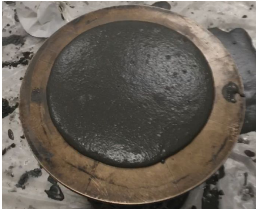
Figure 1. Ultra-high-performance concrete made with Type IL cement during flow testing. Figure: Megan Voss.
