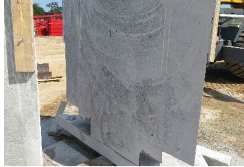
Section cut through pile and footing after mock-up test to demonstrate that concrete could be successfully placed to make the pile-to-footing connection. Photo: WSP USA.
