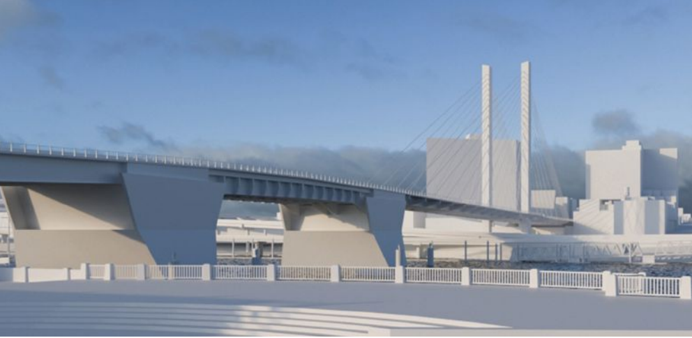
Figure 2. Rendering an engineering model into a photo backdrop creates a more lifelike image of the bridge to share with stakeholders. Because the bridge is shown from the vantage point of a typical viewer, the cables virtually disappear when the actual surfaces of the cables are rendered in the proposed materials.
