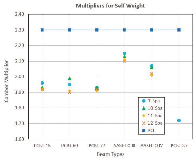
Figure 3. Long-term multiplier to be applied to elastic self-weight deflection at time of transfer for several girder depths and spacings computed using PCI multipliers and a more refined method from PCI Bridge Design Manual .
