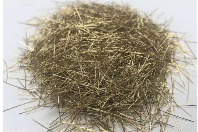
In January 2021, Sumiden Wire began producing 0.2 mm diameter × 13 mm long (0.008 × 0.5 in.) high-strength steel fibers for ultra-high-performance-concrete mixtures. Photo: Sumiden Wire.
