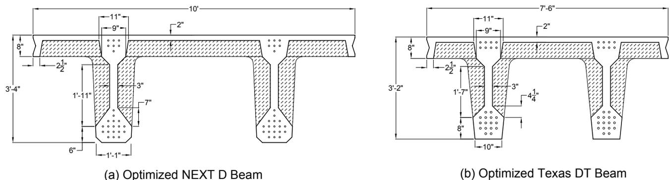
Figure 5. Optimized UHPC shapes for (a) NEXT D beam and (b) Texas double-tee beam based on standard beam shapes with form blockouts. These optimized UHPC illustrative shapes use about 50%–60% of the conventional concrete volume. Figure: e.construct.
