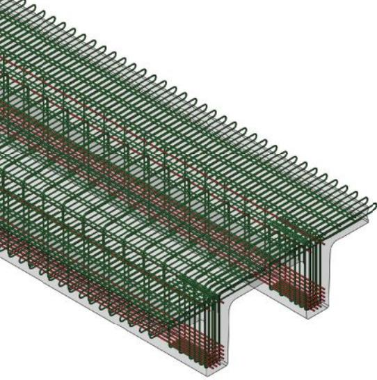
Figure 4. Isometric view of the end of a typical NEXT D beam designed using conventional concrete. Reinforcing bars and prestressing strands are shown. Figure: e.construct.
