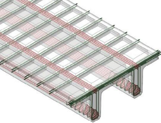
Figure 6. Isometric view of the end of the optimized UHPC twin-stemmed beam from above. Reinforcing bars and prestressing strands are shown. Figure: e.construct.
