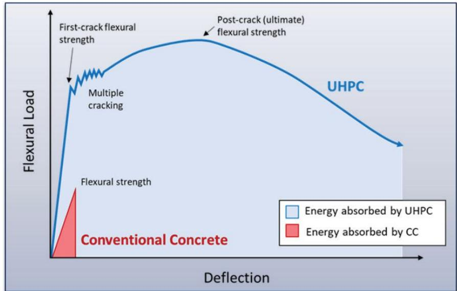
Figure 2. The schematic comparison test results according to ASTM C1609 *Standard Test Method for Flexural Performance of Fiber-Reinforced Concrete*<sup>4</sup> shows much higher tensile strengths and greater ductility for ultra-high-performance concrete (UHPC) than for conventional concrete (CC). Figure: e.construct.
