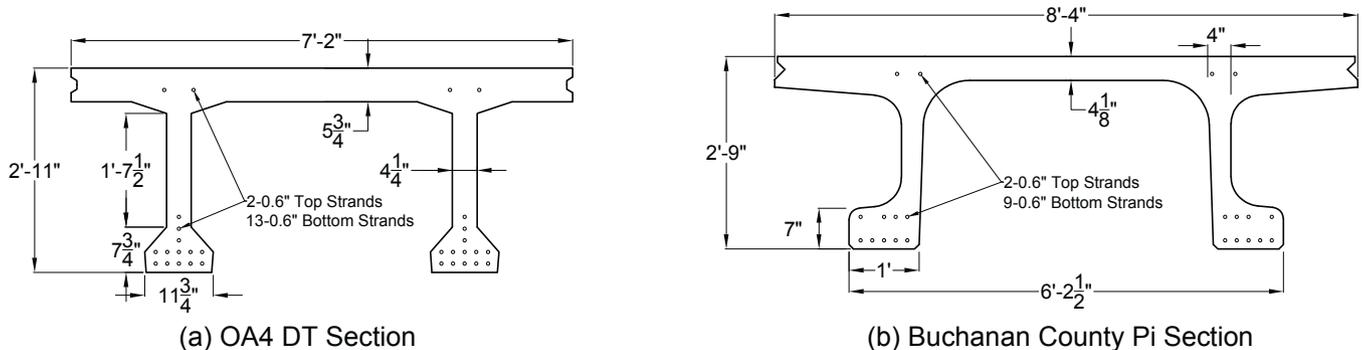
Figure 1. Cross sections for (a) π-shaped beam in France<sup>1</sup> and (b) π section in Buchanan County, Iowa.<sup>2,3</sup> Figure: e.construct.
