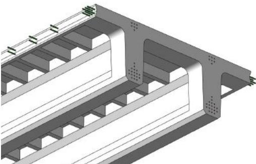
Figure 7. Isometric view of the end of the optimized UHPC twin-stemmed beam from below showing the ribbed deck and solid end block. Figure: e.construct.
