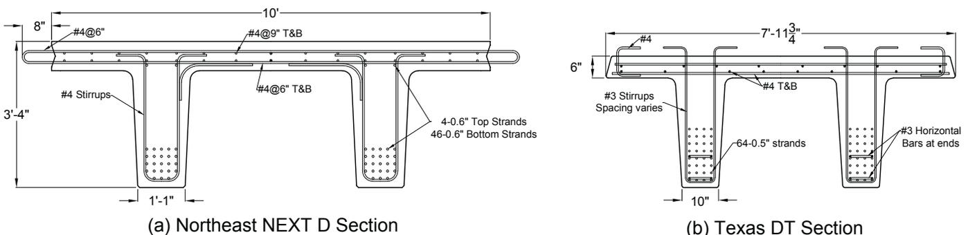
Figure 3. Standard sections for (a) NEXT D and (b) Texas double-tee beams. Figure: PCI Northeast and Texas Department of Transportation.
