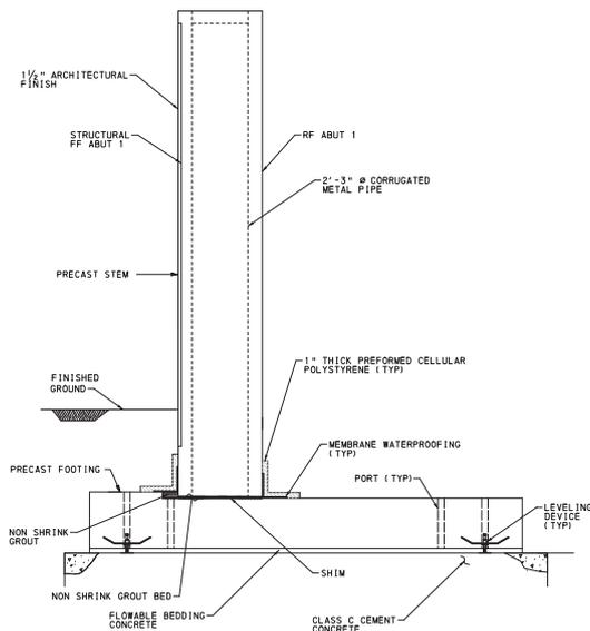
Typical section of State Route 183 precast concrete stem piece at abutment. The 2-ft 3-in.-diameter corrugated metal pipe was used in stem pieces of two bridges to keep the piece weight within the 50-ton limit. Figure: Alfred Benesch & Company.
