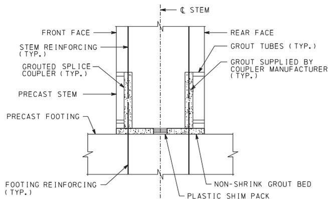
Grouted splice-coupler connection detail between precast concrete footing and precast concrete stem. Figure: Alfred Benesch & Company and Johnson, Mirmiran & Thompson.
