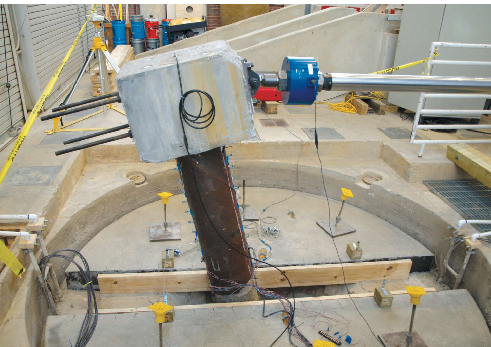
Deformation of reinforced-concrete-filled steel tube during test in soil. Photo: Diego Aguirre.
