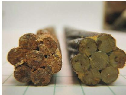
Salt spray testing on untreated and impregnation-treated strands.
