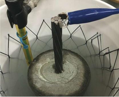
Grouted post-tensioning strand sample undergoing potentiostatic testing.
