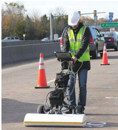
Ground penetrating radar technology being evaluated under the R06A Nondestructive Testing for Concrete Bridge Decks project. Photo: Rutgers University under SHRP2 contract, 2013.
