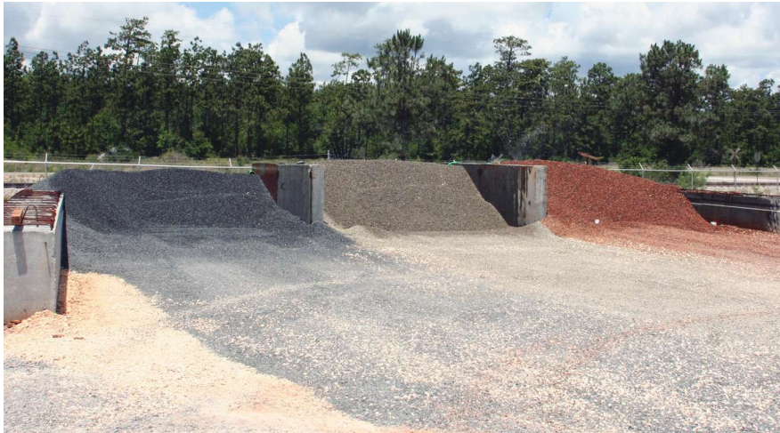
Lightweight aggregate stockpiles at precast concrete plant. All Photos and Figures: FHWA.
