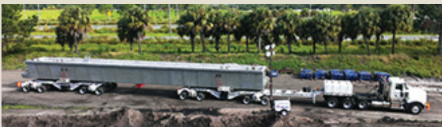
9a) As it arrives at the jobsite, the length of the truck and trailer is 150 ft. Photo: Dura-Stress Inc.
