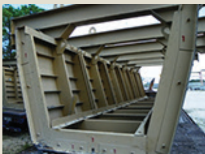
8a) Section of interior bucket form for casting trapezoidal U-girder.
