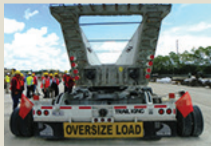
9c) The trailer's axles extend laterally on command to 19 ft out-to-out. This enables the load to travel in two lanes when crossing structures. Photo: J Dick Precast Concrete Consultant.
