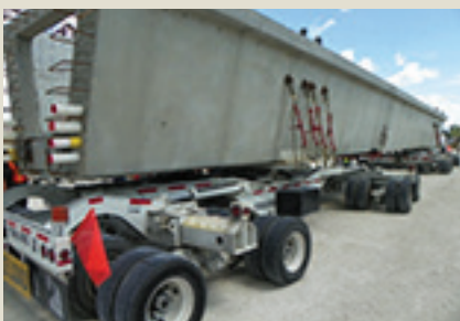
9b) The steerable dollies of the trailer visible at right center. Photo: J Dick Precast Concrete Consultant.
