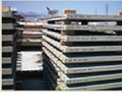
14b) Observed during TechnoQuest 1, precast lid slabs are stored in the precast plant awaiting delivery. Photo: PCI.
