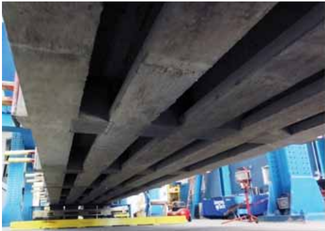
A scaled model of a deck bulb-tee bridge, 40 ft long and 14 in. deep, is shown in the structures laboratory of Lawrence Technological University and following testing to failure. The bridge uses carbon fiber prestressing strands, all nonmetallic reinforcement, and UHPC in the longitudinal joints. Photo: Lawrence Technological University.
