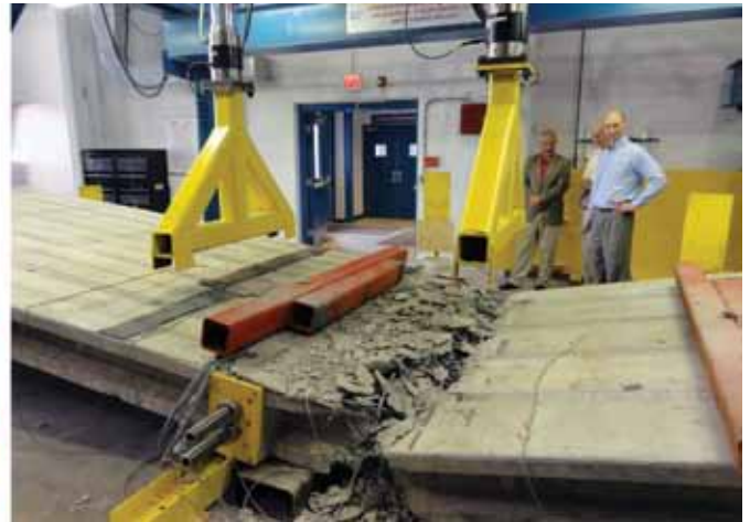
A scaled model of a deck bulb-tee bridge, 40 ft long and 14 in. deep, is shown in the structures laboratory of Lawrence Technological University and following testing to failure. The bridge uses carbon fiber prestressing strands, all nonmetallic reinforcement, and UHPC in the longitudinal joints. Photo: Lawrence Technological University.
