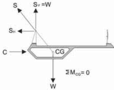
Ideally, the line of action of the suspenders should pass through the center of gravity of the section to achieve equilibrium for dead loads.
