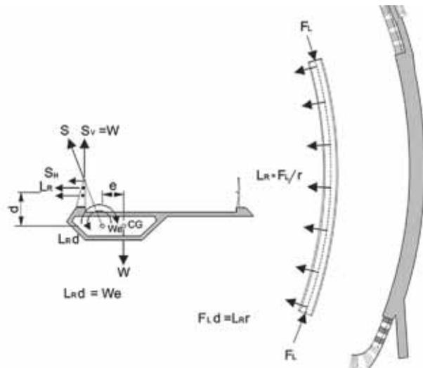
An additional longitudinal tendon was stressed at the top of the railing. Coupled with the curvature of the bridge, this tendon creates an inward radial force to provide the restoring torsion needed for equilibrium.
