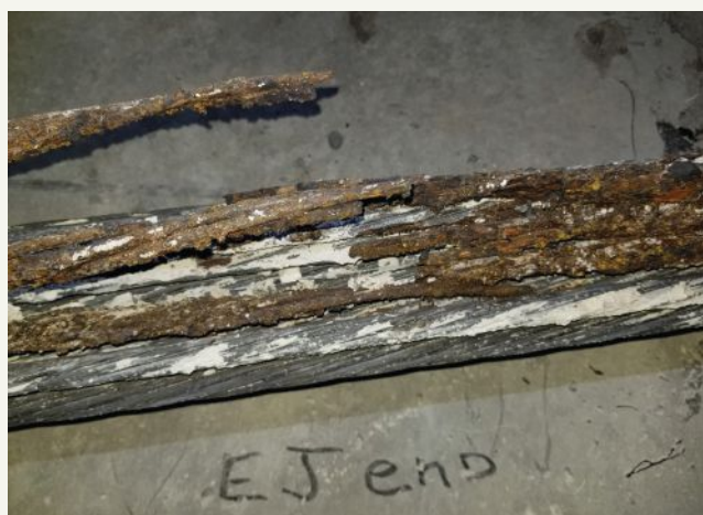
Figure 2. Corrosion of individual post-tensioning strands in an external tendon at a location where the duct was not completely grouted, leaving strands unprotected. Photo: Structural Technologies.
