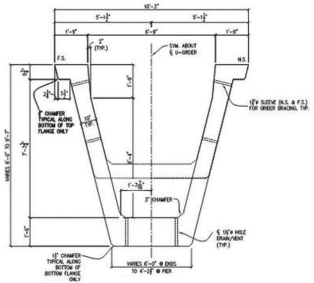
Over-the-road shipping constraints had to be carefully considered due to the 150 ft span and 1200 ft radius of the precast concrete segments. Size limits for hauling the curved precast concrete segments were 14 ft maximum width and 135 ft maximum length. Segments were shipped approximately 20 miles from Leesburg, Fla., to the project site. Cross section of haunched U-beam at the pier is shown at right. Photo: A<sup>2</sup> Group Inc. Figure: Atkins.
