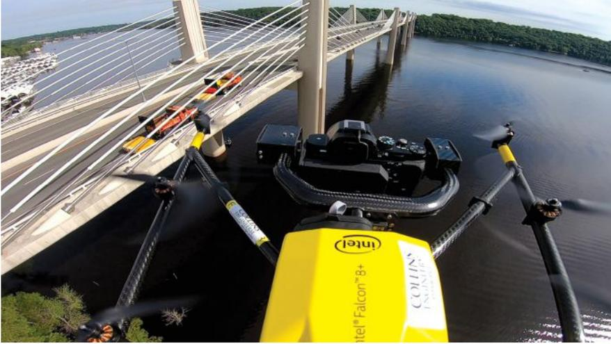
Minnesota Department of Transportation (MnDOT) is one of many agencies employing drones as a way of innovating for a better outcome in its bridge inspection practices. MnDOT inspectors can conduct significant parts of the inspection while in the office. This reduces time in the field, making the overall inspection more efficient, safer, and more cost effective. Photo: Minnesota Department of Transportation.
