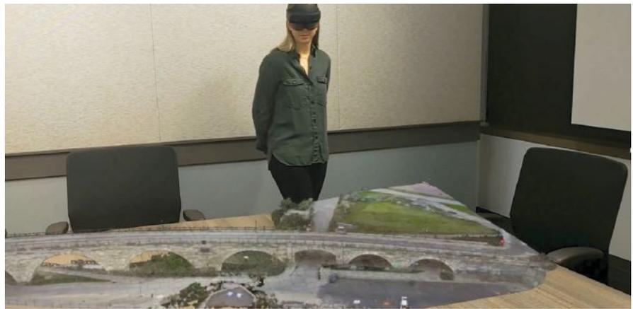
The software company Bentley Systems is adopting Microsoft HoloLens technology so that bridge inspectors can immerse themselves in the full-scale digital model of the bridge they are inspecting. The use of augmented reality aims to improve the connection between the bridge information model and actual field conditions. Photo: Bentley Systems.
