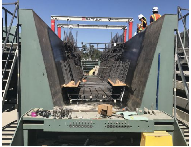
The precast producer used two straight and one adjustable-curve PCI U-96 girder forms. Photo: WSP.
