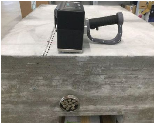
Sonic/ultrasonic impact-echo testing identified potential voids and soft grout areas. See Reference 4.
