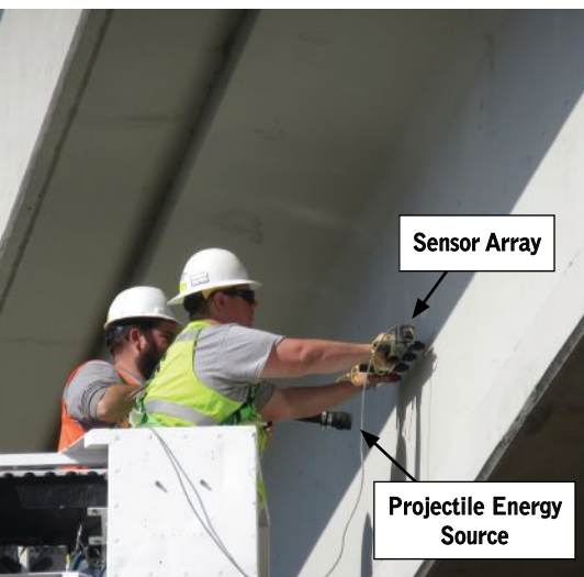
Impact-echo testing. See Reference 2.
