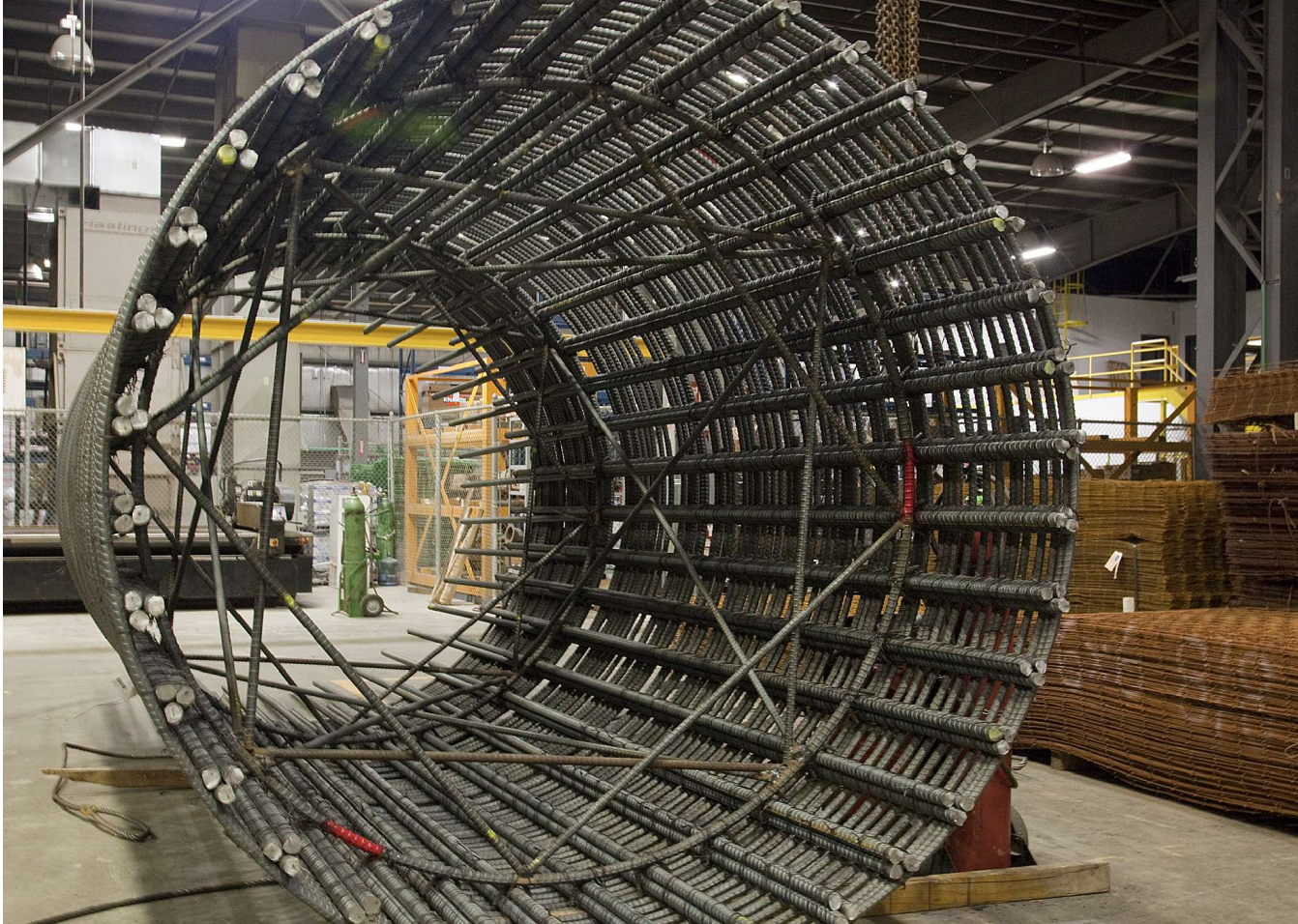
Prefabricated reinforcing cage for bridge column in seismic region with very heavy reinforcement. The Concrete Reinforcing Steel Institute's certification standards for epoxy-coating plants, fabricators of epoxy-coated bars, and fabricators of stainless steel reinforcement help ensure quality products. Photo: Dimension Fabricators Inc.
