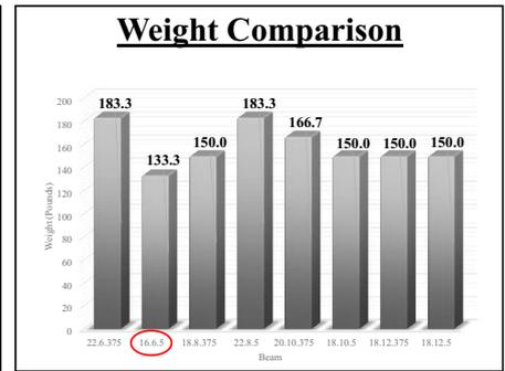
Prioritized optimization criteria: comparison of deflection, cost, and weight at failure [measure of section ductility] for various designs.
