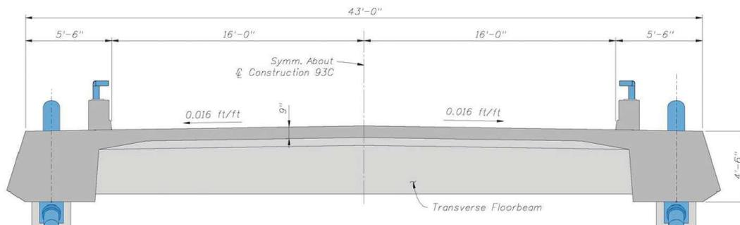
Typical deck section, showing concrete edge girders, transverse floor beams, and deck.
