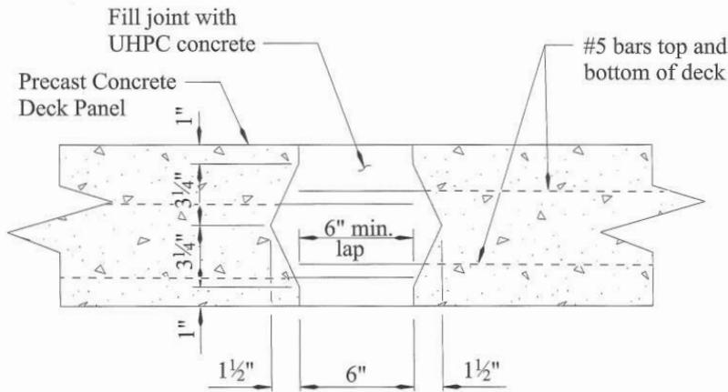
Ultra-high-performance concrete, keyed-joint detail used to connect the precast concrete deck panels for the Burnt River Bridge project. Figure: George Bornstedt.
